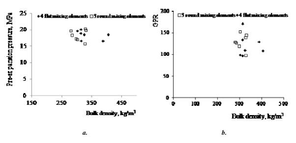
Figure 7. Influence of pre-expansion pressure and GPR on bulk density
