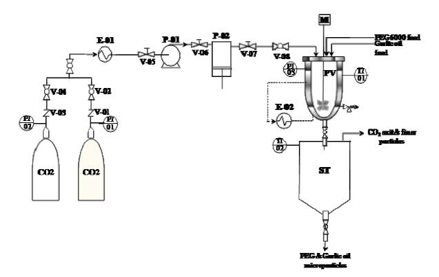
Figure 1. Flow diagram of the batch PGSS process
