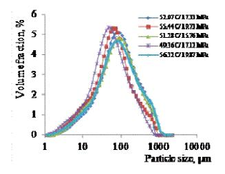
Figure 5. Particles size distribution for powder obtained by PGSS process with 3 round mixing elements
