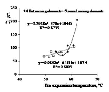
Figure 3. Influence of the pre-expansion temperature on particles size
