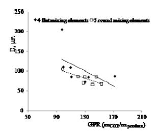
Figure 4. Influence of the gas to product ratio on particles size
