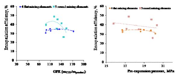
Figure 6. Influence of the process parameters on the encapsulation efficiency
